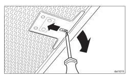
If the filters are incorrectly installed, insert a small screwdriver into the slit along its edge to disengage them from the casing.
